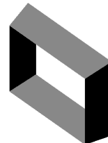
A rectangle extruded as a thin feature, with draft
